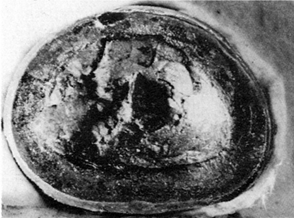
Damage to the base of the Magic Bullet, showing the distorted, flattened shape of the bullet.
